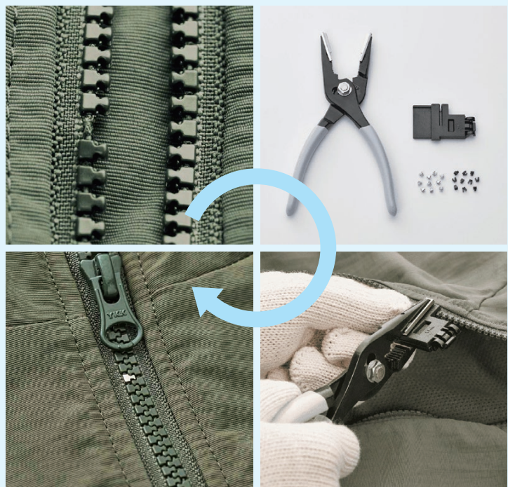
Revived replacement elements for VISLON®. Zippers can be repaired by attaching die-cast revived replacement elements, using a special tool to replace elements that have come off
